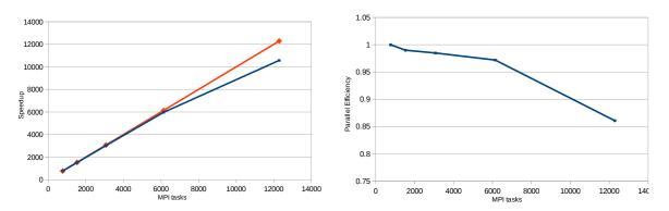
Figure 2: Interface coupling with MUI. 3M data points transferred at each time-step. Speedup (left) with ideal speedup in red. Parallel efficiency (right).
