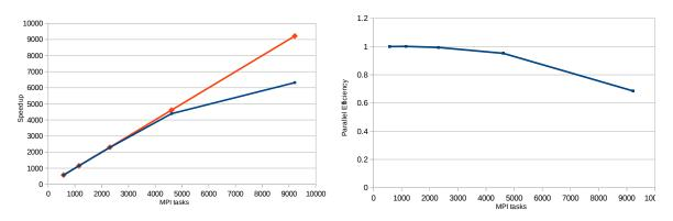
**Figure 1**: Volumetric coupling with MUI. 200M data points transferred at each time-step. Speedup (left) with ideal speedup in red. Parallel efficiency (right).
