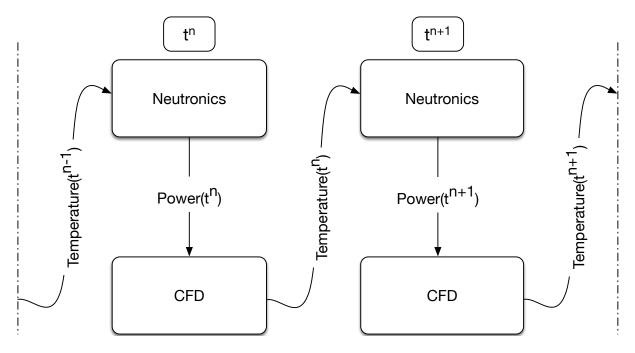
Figure 3: Data communication pattern employed for neutronics-CFD coupling.
