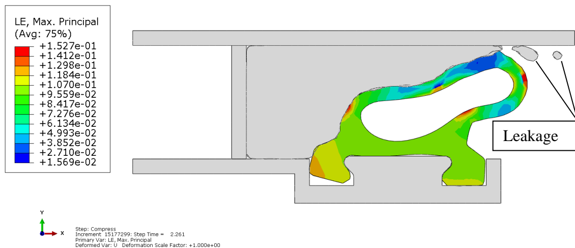
Figure 4: Maximum principle strain of seal under 12.5mm compression during leakage
