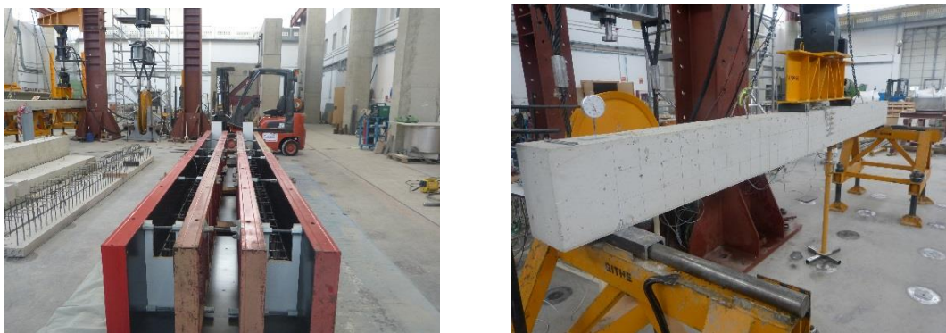
Figure 8: Four-point flexural test carried out at Universidad de Burgos
