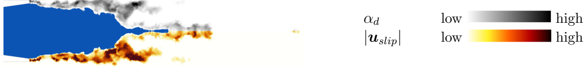
Figure 2: atomized NIR7eq (Legend: blue isovolume of \alpha_2 = 0.99 , slip velocity norm |\mathbf{u}_{slip}| , volume fraction of droplets in the SPIREE solver \alpha_d )
