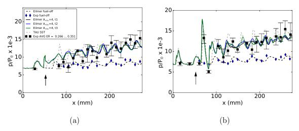
Figure 4: Pressure along the wall at the x-z symmetry plane between the hydrogen injectors. (a) injector side, (b) cowl side.  $P_0 = 17.73$  MPa.
