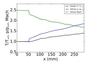
Figure 5: Stream-thrust averaged quantities along the HyShot II combustor.  $A_{\rm edm}=4,\, Pr_{\rm t}=0.9$  ,  $Sc_{\rm t}=0.7.$
