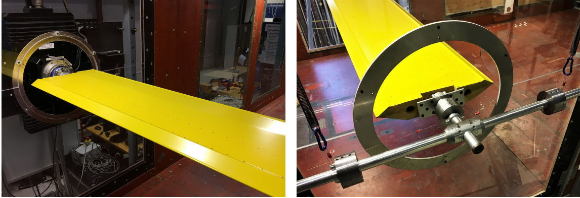
Figure 5: The Hardanger bridge deck sectional model installed for forced-vibration (left), and free-vibration wind tunnel experiments (right).
