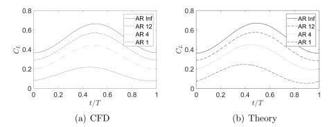
Figure 4: Coefficient of lift comparison for baseline cases.
