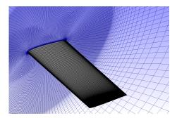
Figure 3: Close-up of computational mesh.
