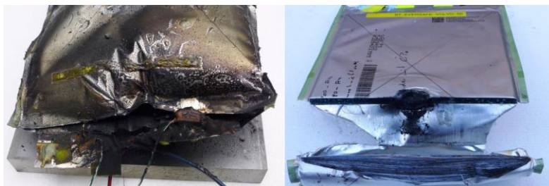
Fig.2: Different reactions for pouch cell abuse tests: imploded cell after nail penetration (left) and intact cell after cut test (right).
