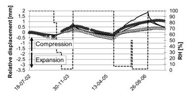
Relative displacements between the tunnel wall and an anchor point 2m inside the rock mass. Observed and computed results
