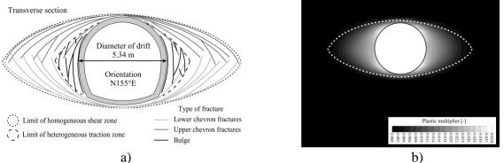
Excavation damaged zone a) Observed [1] b) Computed
