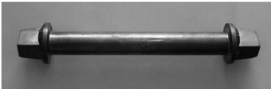
Fig. 4: The forging formed in three-slide forging press
