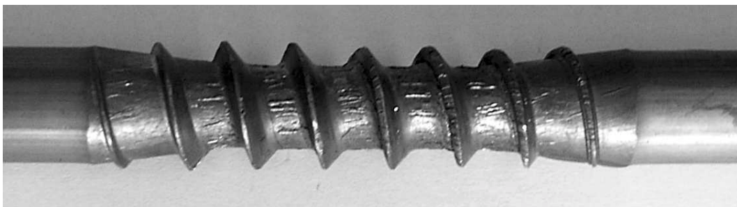
Fig. 2: The thread rolled on lead billet
