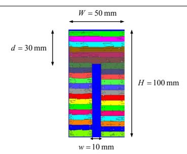
Fig. 3.1 Geometry and initial configuration of the transfer chamber
