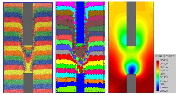
Fig. 3.2 Displacements field and density field after powder transfer stage. Left): experimental distribution of layers after the transfer process, center): numerical distribution of layers and right): density distribution.
