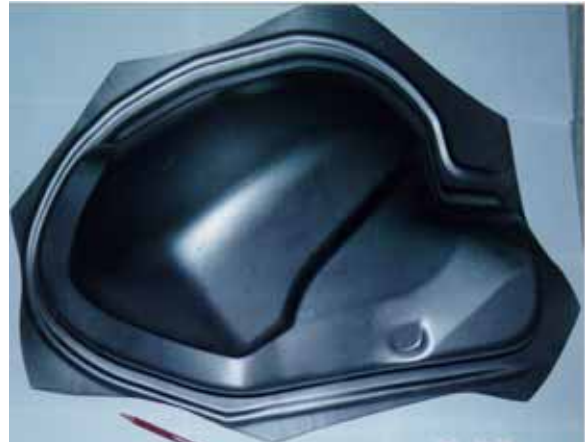
Fig. 5 A sound production part without wrinkles and fracture.
