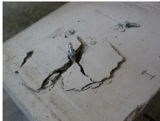
Fig.2 Failure of concrete and rupture of anchor after tension test with couple of anchors
