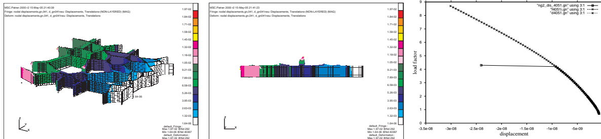
Figure 4: Spatial failure of the interfaces, axonometric view (left) and side view (middle), displacement vs load factor (right).
