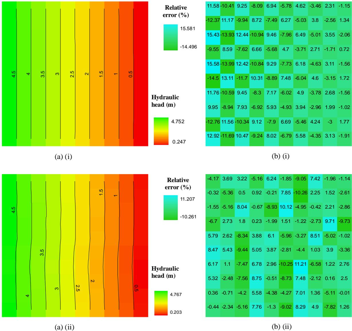
Figure 1: (a) block centered heads and (b) relative errors in top layer impedivities when using 1% noise in (i) west and (ii) top boundary heads
