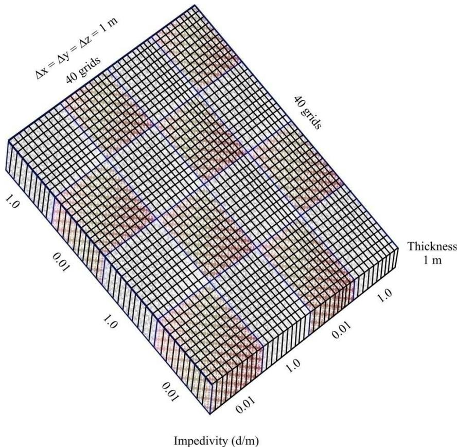
Figure 2: Dimensions of the fine-scale model example 2 with checkerboard impedivity pattern
