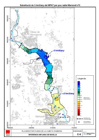
Figure 5. Drawdown map obtained with the improved aquifer-river interaction. The effects are consistent with some pumping tests and data available up to date.
