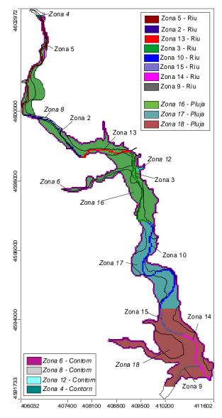
Figure 2. Zonation of the aquifer-river relationship with the former 2004-model, when the river was represented by 10 prescribed recharge zones (coefficients). Aerial rain recharge and lateral flows are also displayed.
