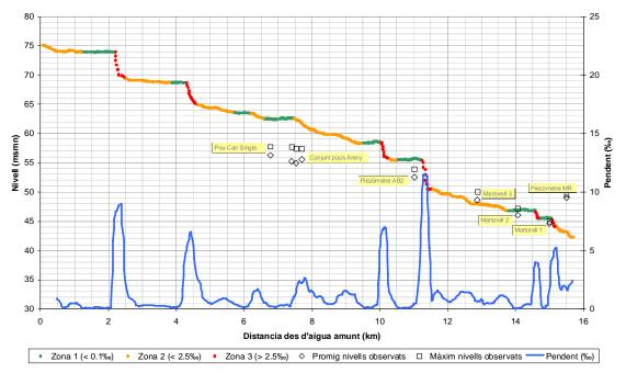
Figure 4. Zonation of the river coefficient depending on the river slope.
