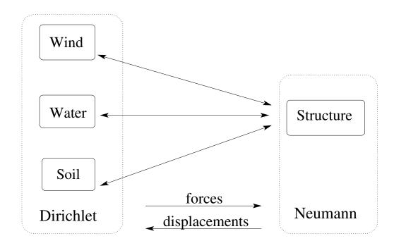
Compared with the parts on the left hand side high density/stiffness of the structural part ==> classical iteration schemes work
