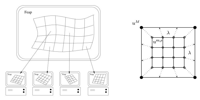
coupling of the displacements using Lagrange-multipliers
