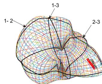
Figure 1 A tri-axial failure surface for a Quasi-Isotropic layup under [1,2,3] loading directions. The surface is calculated from the multiscale frame work here. Red circles show the meso-scale RVE results.
