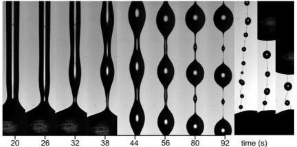
The formation of the beads-on-a-string structure during the capillary break-up of a droplet of saliva. The time elapsed from the formation of the cylindrical filament is indicated. The filament remained stable for minutes and final rupture has been initiated by agitating the system. This is shown in the three photos on the right that show the stiffness of the polymeric fiber that is formed between the remaining droplets.
