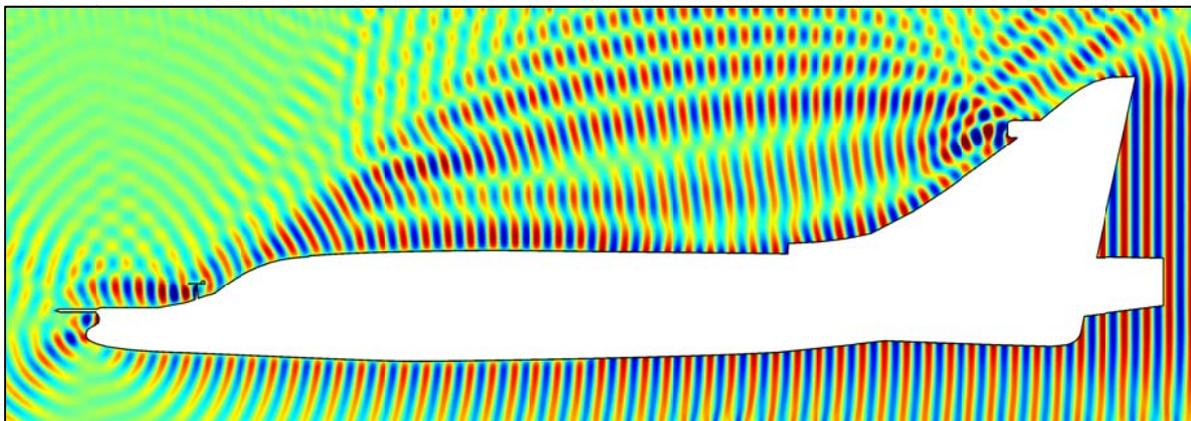
**Figure 1.** Scattering of an electromagnetic wave by a complex geometric configuration containing small geometric features.
