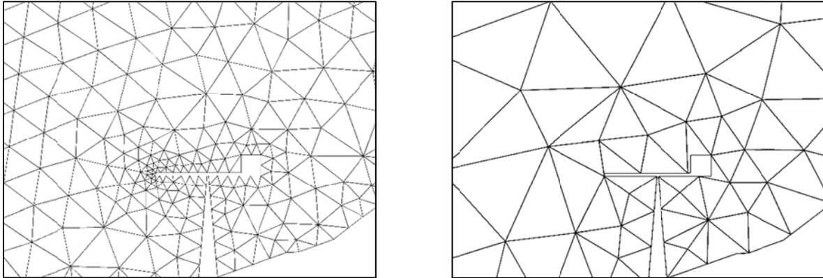
**Figure 2.** Mesh produced with a standard FE mesh generator (left) showing the required mesh refinement to capture small geometric features and mesh produced with the new approach (right) showing coarse elements capturing complex boundary geometric features.
