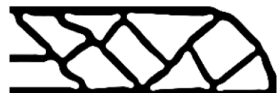
Fig. 3: Maximum / minimum size control and separation distance.
