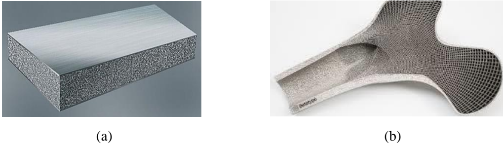
Figure 1 Monolithic sandwich-like parts with porous cores: (a) regular shape and (b) irregular shape.
