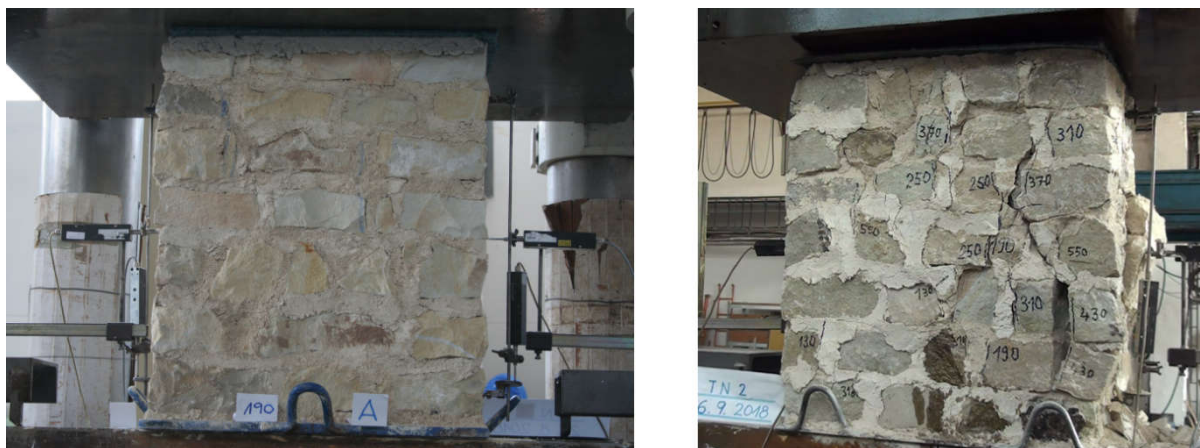
Fig. 1 Test specimens of multi-layer masonry segments before and after experimental loading.
