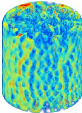
Figure 1 : Velocity field over beads network
