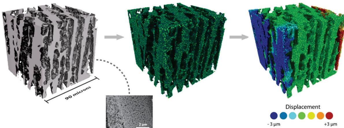
From an X-ray tomography reconstructed volume to a DEM simulation of crushing strength.
