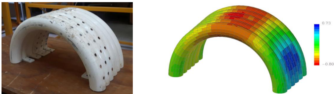
Figure 1: The model of the open structure for the wind tunnel tests (on the left) and the pressure coefficient field when the wind blows from the right (on the right)
