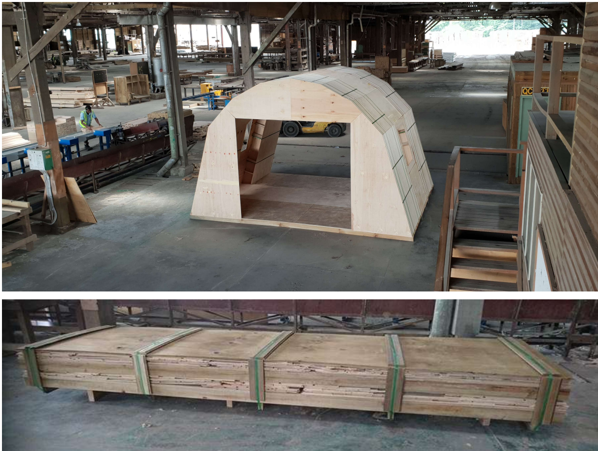
Figure 1: 20m 2 ‘Plate House’ transitional shelter prototype, constructed February 2019. Top: erected structure. Bottom: packaged kit-of-parts.
