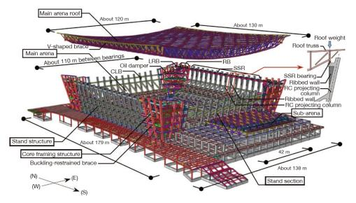
Structural Diagram of Main Arena and Sub-arena
