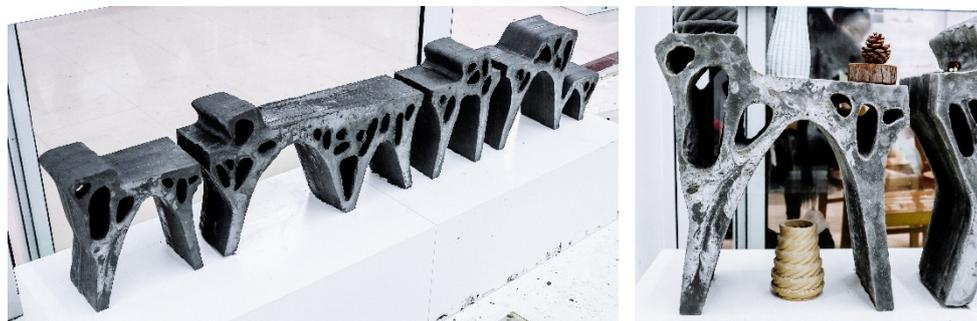
Figure 1, Topology optimized concrete components fabricated via clay mould technology.
