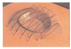
The structure principle 2 is called the "arch-ridge-valley roof". The principle is the tightening of a mat of cables between a series of crosswise running rigid arches, alternately curved hill like and valley like. The steeply inclined north facing surfaces carry the windows, the gently sloped carry the thermally insulating panels. The arches which support the cable net are supported by trestle-systems at the outer edges of the hall.
