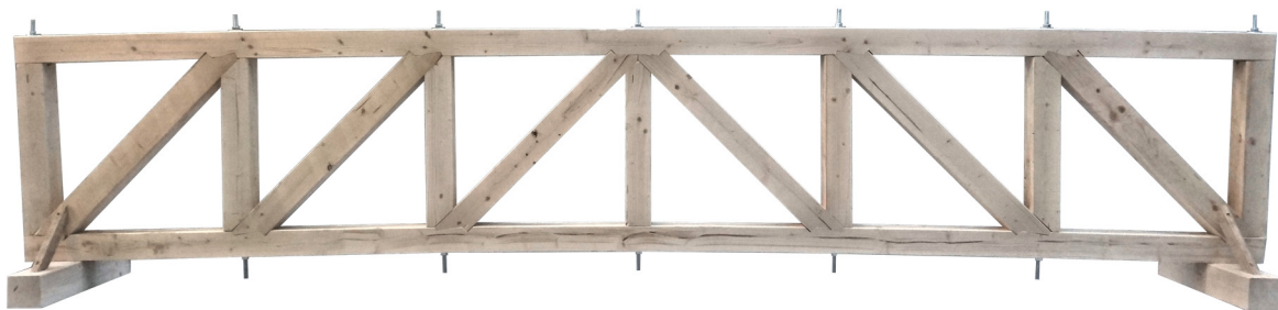
Figure 1: Specimen 1, superelated truss with the help of shortening or lengthening their lacings depending on the subjected load with a span length of 4.80m
