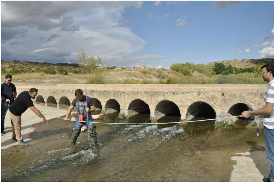
**Figure 1:** Students measuring flows and dimensions in a river channel during the fieldwork
