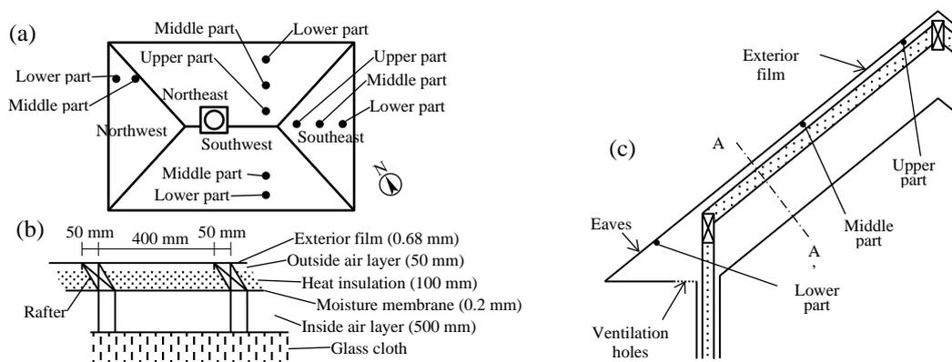
**Figure 1.** Measured house: (a) roof plan, (b) A–A' section of roof in (c), and (c) vertical section of the roof.
