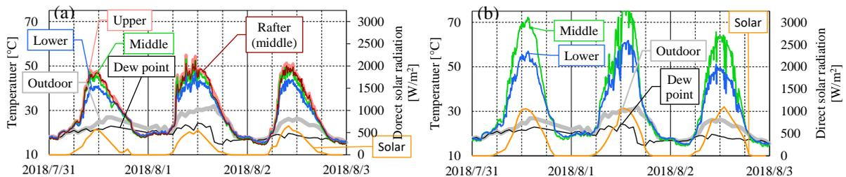
**Figure 3.** Direct solar radiation and surface temperatures of (a) northeast and (b) southwest roofs in summer.
