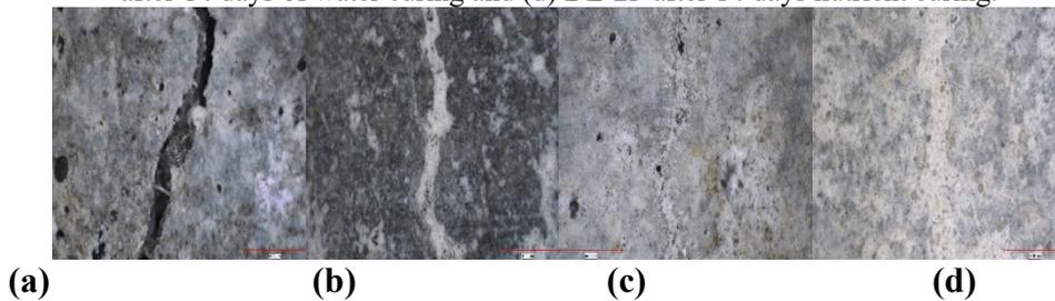
**Figure 2.** Stereomicroscopy images of the cracks (0.3 to 0.4  $\mu\text{m}$ ) in 28-day old specimens containing pumice (a) Pum-Bac after 28-days of water curing (b) Pum-Bac after 28-days of nutrient curing (c) Pum-2P after 14-days of water curing and (d) Pum-2P after 14-days of nutrient curing.
