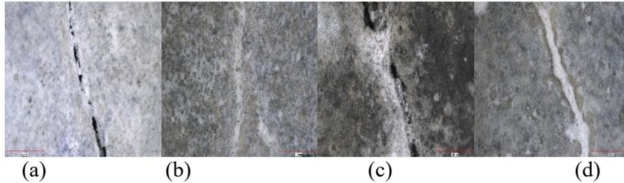
**Figure 1.** Stereomicroscopy images of the cracks (0.3 to 0.4  $\mu\text{m}$ ) in 28-day old specimens containing diatomaceous earth (a) DE-Bac after 28-days of water curing (b) DE-Bac after 28-days nutrient curing (c) DE-2P after 14 days of water curing and (d) DE-2P after 14 days nutrient curing.
