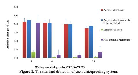
It is noted that the behavior of the bituminous and polyurethane systems proved to be very sensitive to temperature and wetting cycles. It is noticeable that the bonding of the bituminous sheet is the lowest among the other systems, even when it is in cycle 0. When in cycle 0 the resistance of the polyurethane system was considerably elevated concerning the other systems, but throughout the cycles of weathering, it lost this initial behavior.
