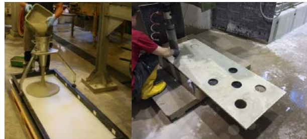
Figure 2. Concreting of test samples (left) and core extractions (right) to assess the self-cleaning properties.
