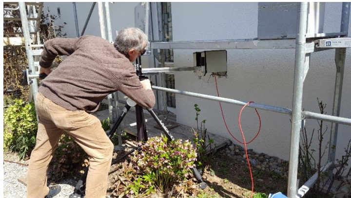
Figure 2. On-site determination of the hail resistance with an ice ball launcher
