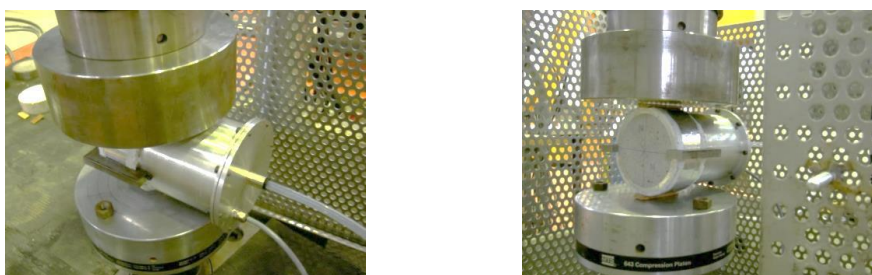
Figure1: Permeability analysis while performing a Brazilian test on a mortar sample. [5]
