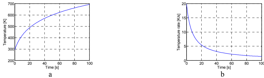
Fig. 8 - ISO 834 time - temperature curve: a) time vs. temperature; b) time vs. temperature rate
