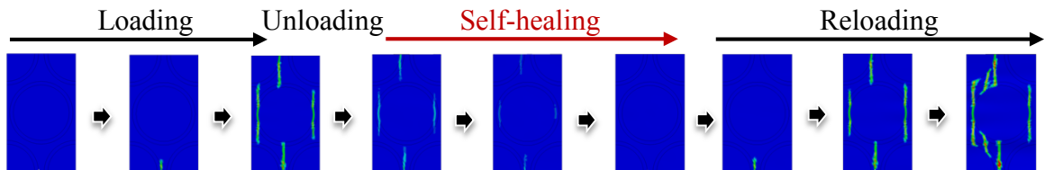
Figure 6: Contour map of damage variable during cyclic loading in the case of high healing velocity condition.
