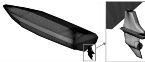
Figure 3: CFD model of Numerette with detailed view of the sterndrive
