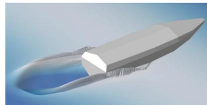
Figure 4: Predicted free surface elevation for captive simulation at sea state 3 most probable wave condition and  $Fr=2.9$
