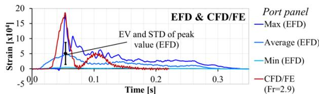
Figure 3: Average, min and max of EFD (Experimental Fluid Dynamics) strain with its expected value (EV) and standard deviation (STD) at peak compared with CFD/FE predicted strain.
