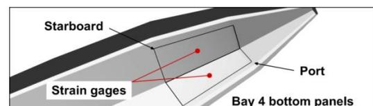
Figure 2: Bottom panels and strain gage location
