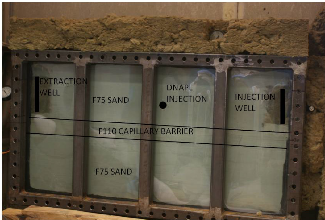
Figure 1: Laboratory scale tank simulated
